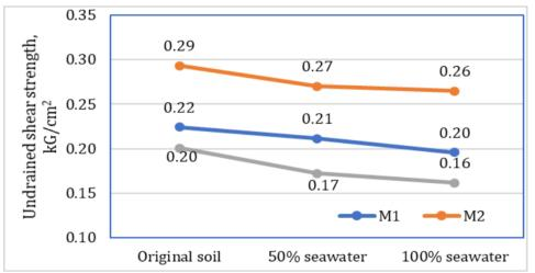
Figure 8. Variation of undrained shear strength of soil after soaking in different salt solutions.
