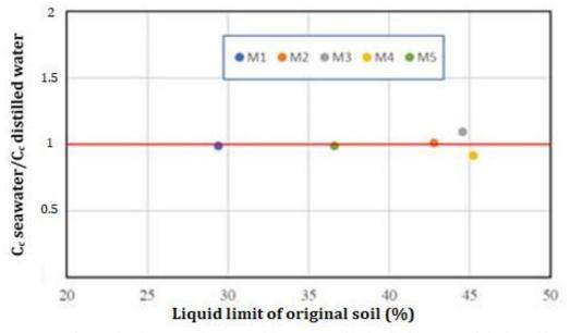
Figure 6. Relationship between the ratio of  $C_c$  seawater/ $C_c$  distilled water and the liquid limit of the original soil.
