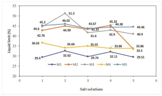
Figure 2. The variation of the liquid limit in different salt solutions.
