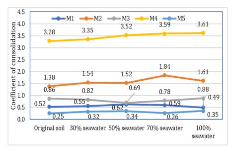
Figure 7. Variation of the vertical coefficient of consolidation (Cv) after soaking in different seawater solutions.
