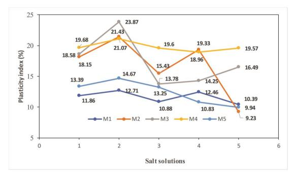
Figure 3. Variation of the plastic limit of soil in different seawater solutions.
