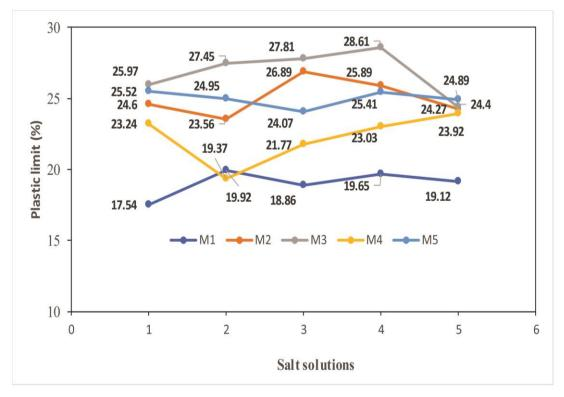
Figure 4. Variation of the plasticity index of soil in different seawater solutions.
